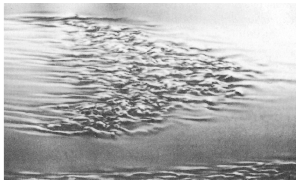
Figure 9.13 (p. 483) Turbulent spots and the transition from laminar to turbulent boundary layer flow on a flat plate. Flow from left to right. (Photograph courtesy of B. Cantwell, Stanford University.)
