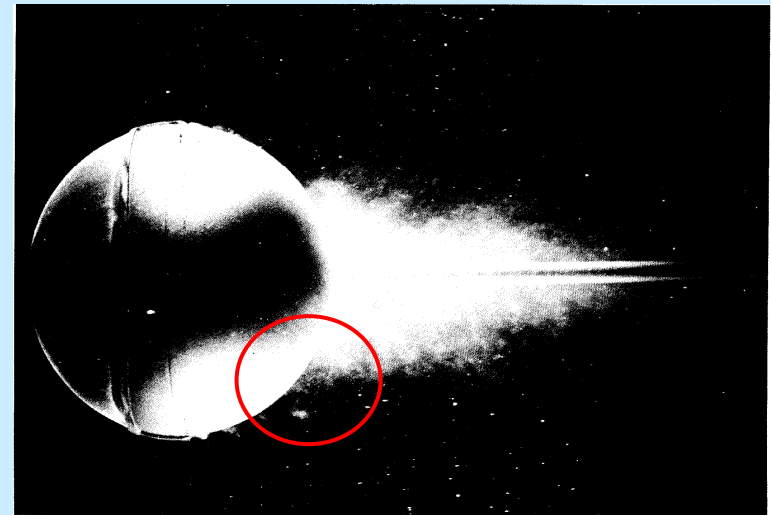
57. Instantaneous flow past a sphere at R=30,000 with a trip wire. A classical experiment of Prandtl and Wieselsberger is repeated here, using air bubbles in water. A wire hoop ahead of the equator trips the boundary layer. It becomes turbulent, so that it separates farther
